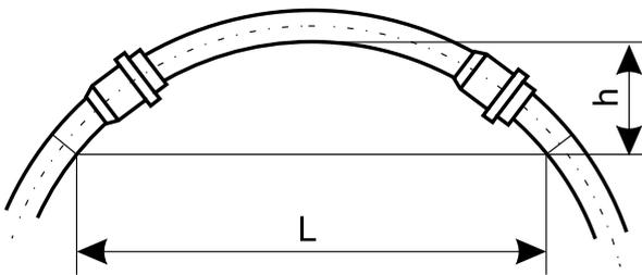
(Bending of pipes > DN 200 is practically impossible in view of their greater intrinsic rigidity)
