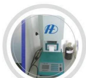
Melt Flow Rate Instrument
