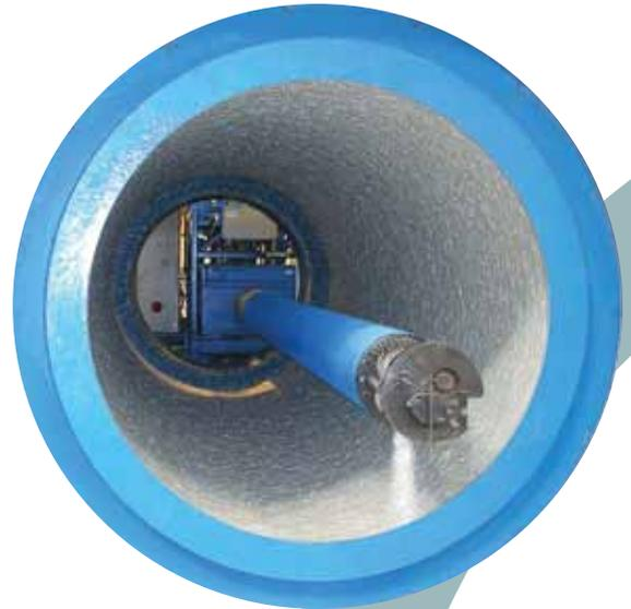
**Centrifugal casting process patented by HOBAS**
