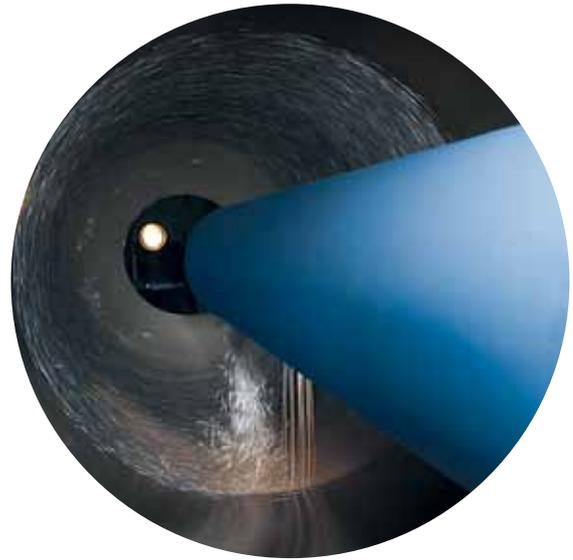
**Centrifugal casting process patented by HOBAS**
